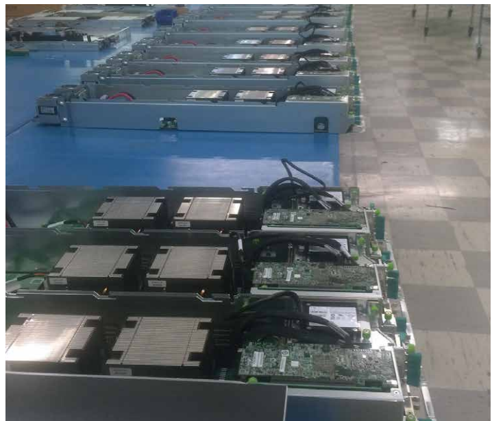
Assembled OCP server awaiting shipment
