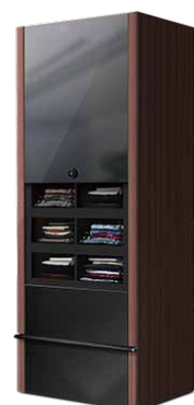
The “Laundroid,” which folds and sorts washed and dried laundry Photo courtesy of Seven Dreamers
