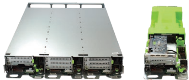
The Wiwynn OCP server is a product with a simple structure. Parts can be replaced without the use of screw drivers and other tools.
