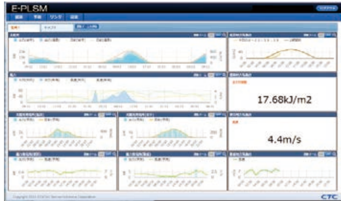
Dashboard that allows users to monitor output and weather conditions (in this case wind volume) at renewable energy power plants
