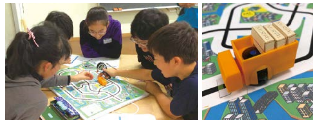
Children are fascinated by Ozobot as it runs automatically along lines traced on a map.
